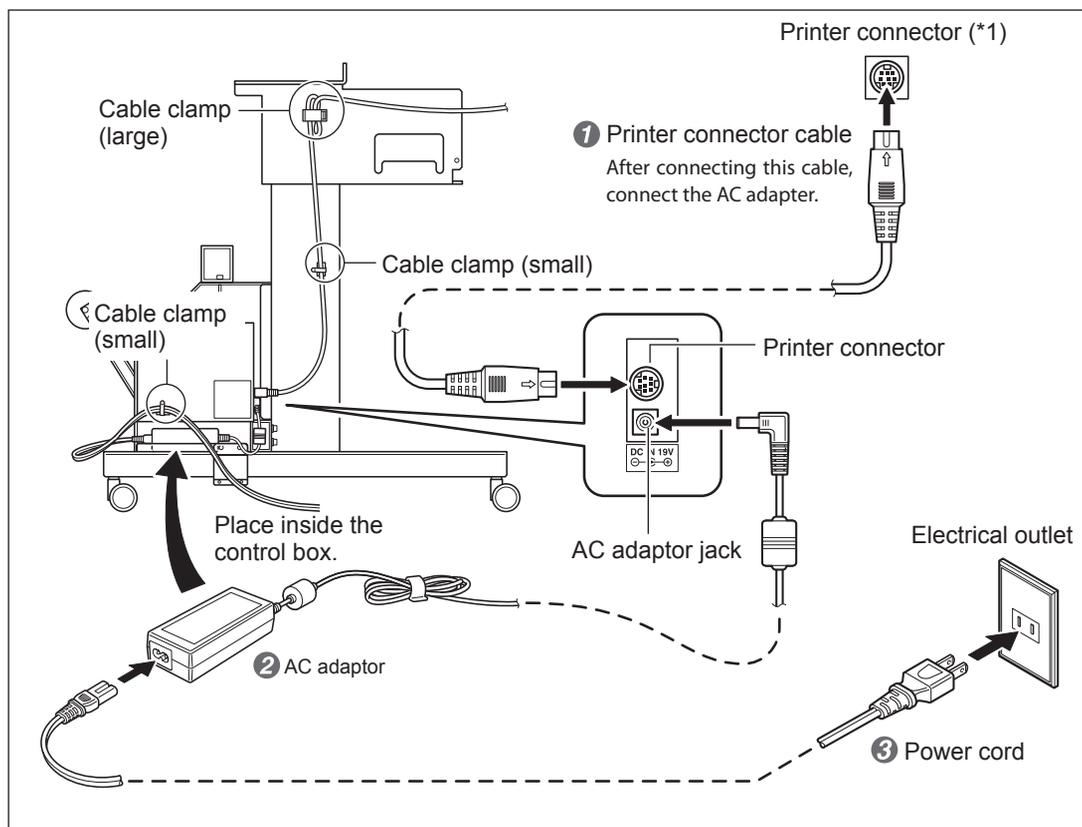
(\*1) The position of the printer connector differs depending on the model. On the VG series, the connector is located on the front of the printer, below the heater. On the VS series, the connector is located on the back of the printer, close to the power supply.
